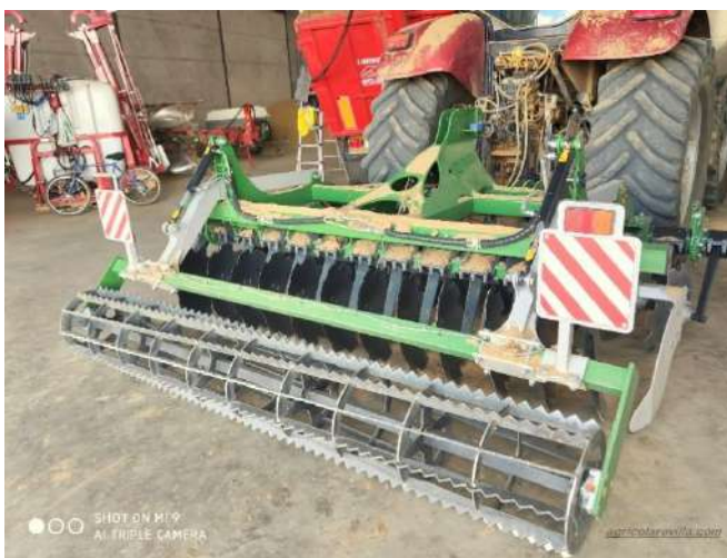
Imatge 12: Grada. FONT: https://www.agricolarevilla.com/wp-content/uploads/2021/09/Grada_rapida_Tolmet_1dsw34-400x300.jpg
